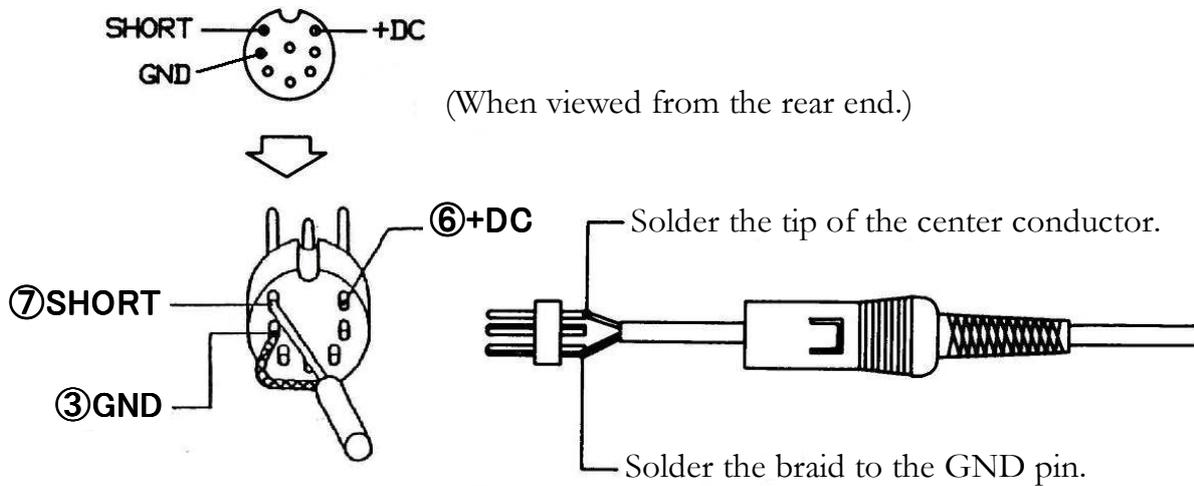
\*Note: If the transceiver externally supplies no voltage (0V, =TX Gnd.) during the TX, solder the center conductor to Pin⑦ (SHORT), or if it supplies positive DC voltage of 2 to 15 V, then solder to Pin⑥ (+DC).
